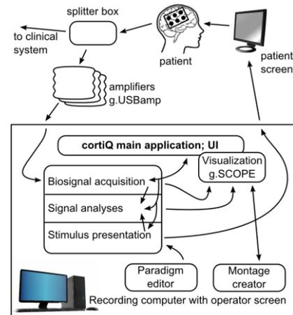
Figure 1: Hard- and software architecture of the cortiQ system.
